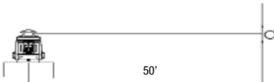
7. If point C and point D are within 1/32" at 50', the accuracy is within tolerance.
